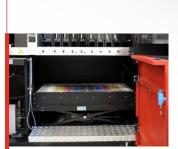
SCISSOR LIFT ON DIP TRAY A scissor lift right underneath the printing heads lowers the dip tray for more convenient cleaning.
